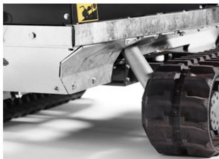
Ground clearance of 220 mm, easy service and reinforced hose protection. Variable track width 1000-1400 mm
