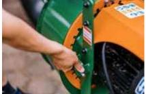
In just a few steps, the pressure joint can be adjusted by a total of 270 °.
