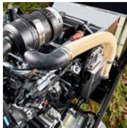
Hatz 4H50 Stage V motor van 55,0 kw
