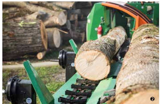
Constant supply of the log feeding system consisting of 1 cross conveyor and 2 longitudinal conveyor.
