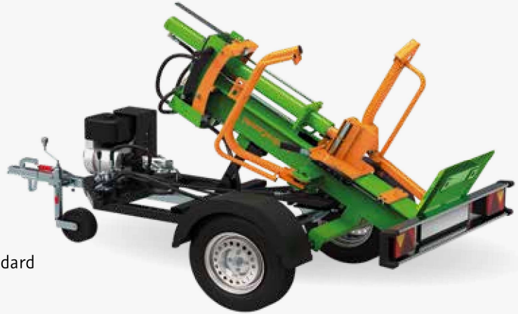
HydroCombi 13 chassis B5.5 D-V2, transport position
