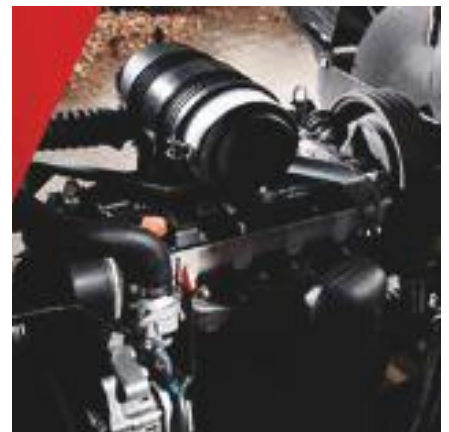
Hoog koppel - minder trillingen 4 cil. Kohler stage V-motor
