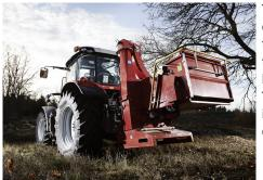
TP 250 PTO is equipped with a folding funnel with the operating bar hinged at the top. The ejector spout is rotatable (300 degrees).
