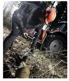
Optional equipment: The TP WINCH is driven by the wood chipper's hydraulic system. The winch pulls in the trunks, making the work even easier and more work environmentally friendly.
