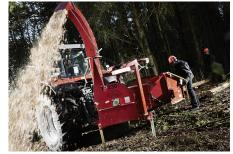
As for all TP Wood Chippers, TP 230 PTO is simple to service; all wearing parts can be changed with standard tools. For maximum safety, there is a disc lock while changing blades.
