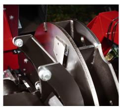
**TP OPTICUT<sup>™</sup>:** The divided blade system ensures that there is always a blade engaging the wood. The result is less vibration, a more steady strain on the machine, lower fuel consumption level and a more uniform wood chip quality.
