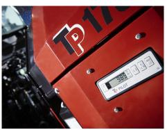
**TP PILOT<sup>™</sup>:** The main purpose of the stress control system is to prevent the tractor from overloading. Likewise, the system enables monitoring of the speed of rotor disc and feed rollers. The system also includes an hour meter.
