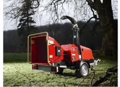
TP 175 MOBILE is mounted on a one-axle galvanized trailer with overrunning brake system and stabiliser.
