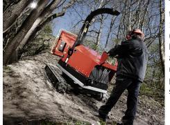
The low caterpillar treads makes TP 160 TRACK ideal for uneven ground. The low caterpillar treads are adjustable for a narrow or wide belt position and have two speeds.
