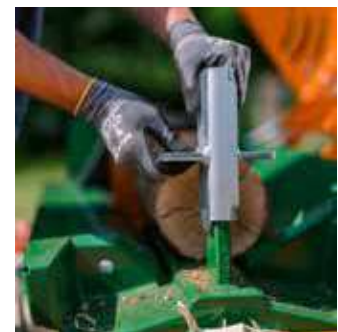
Oscar: The optional 4-way reversible splitting wedge can be used on both sides for various diameter logs.
