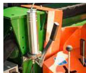
Integrated lubrication device with hand pump (optional).
