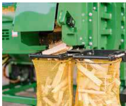
The movable double frame for loosely packed mesh bags.
