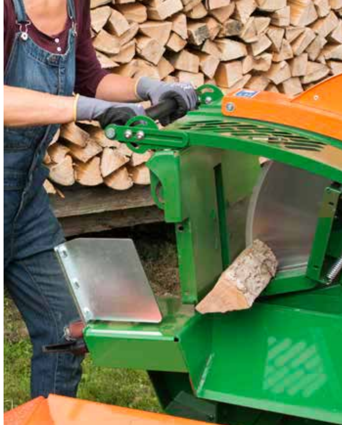
Safety flap with ergonomic height adjustment: The danger area is covered.
