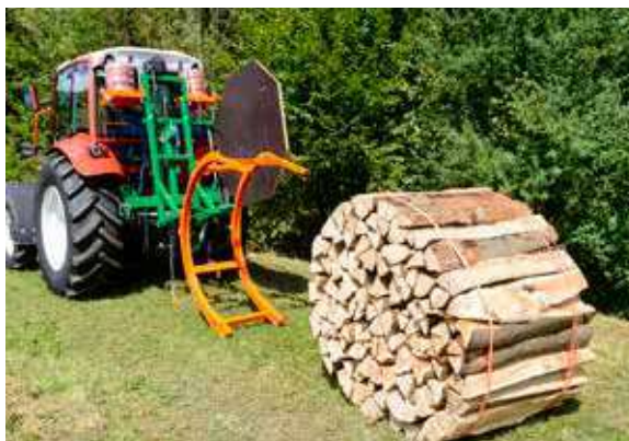
The ready-tied bundle can be conveniently rolled out of the bundling device.
