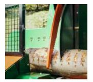
The WIDIA carbide saw blade with 100 cm Ø shortens the log to 20 to 50 cm and is particularly long lasting. The hydraulic log downholder safely retains the logs during the cutting process.
