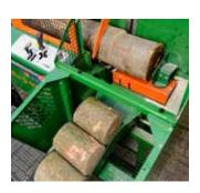
The cut log section is passed on to the AutoSplit via the hydraulic ejection rocker and the log chute. The optional buffer belt is an ideal additional solution for the fast transportation from the sawing unit to the splitting unit.
