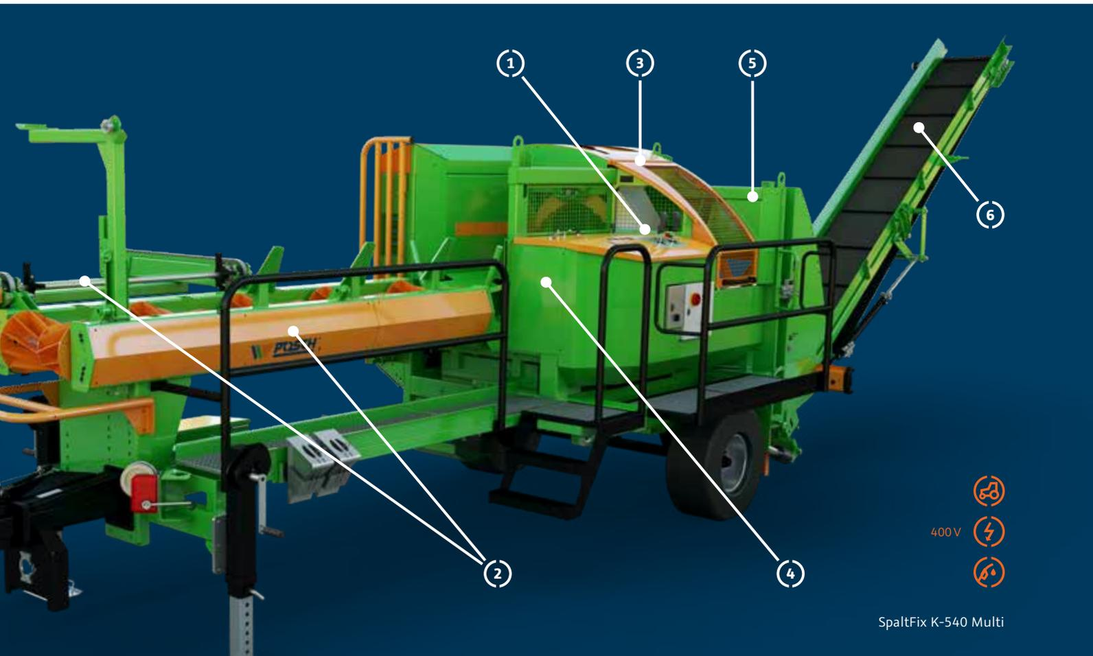
**3 SuperCut Harvester saw for fast and safe cutting**
