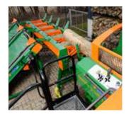
The logs are transported to the sawing unit via the powerful feed belt. Log support systems comprising longitudinal and cross conveyors can be combined individually depending on the requirements.
