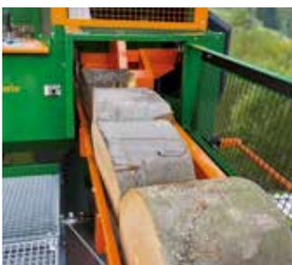
The hydraulic ejection hatch and the standard buffer belt ensure smooth transportation of logs to the splitting process.
