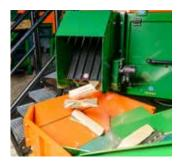
For firewood with a length of 12–33 cm, the billet edge length can be adjusted variably from 4–15 cm. For optimum kindling with a length of up to 20 cm, finer billets are possible too.
