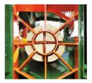
The hydraulically adjustable MULTI splitting knife produces an optimum result with every log diameter.
