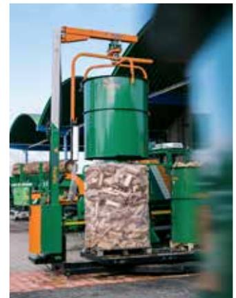
As soon as the filling drum has been pulled up all the way, the mesh is severed and the pack of billets is carted away.
