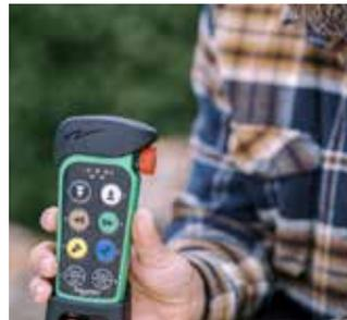
You control all functions comfortably via radio remote control. At the push of a button, you can move the wood from the AutoFeed to the sawing unit or start the sawing and splitting process.
