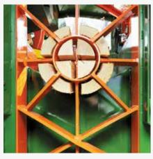
More options without knife change. The hydraulically adjustable frame knife adapts to the log diameter and produces up to 18 billets per cycle without knife change.
