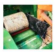
The entire log section is transported to the splitting punch via the hydraulically operated wood rocker. The punch pushes the log against the splitting wedge.
