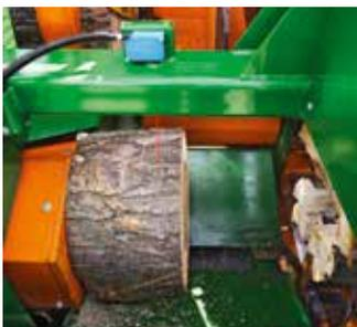
The pressure piece presses the timber with 35 t against the double-edged splitting knife and so quickly produces the maximum number of billets.
