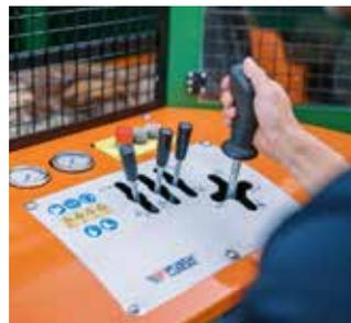
Whole logs with a thickness of up to 70 cm are easily and carefully passed on to the PowerCut sawing unit and cut there according to the length settings. With the clearly structured control panel, it is easy to control all processes.
