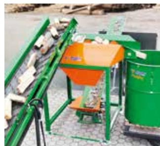
The conveyor belts transport the finished billets to the respective packaging solution. The combination of the timber cleaner LogFix and the PackFix system produces firewood of high quality and in neat packages.
