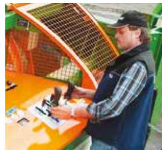
With the 2-hand joystick on the clearly structured control panel, it is easy to control all processes. The log manipulator is used to put the logs in the right position before processing.
