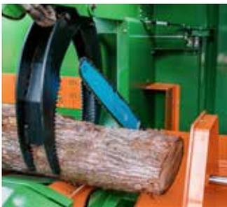
New: SuperCut harvester unit with longer sawbar life cycle and easier chain and bar swap, improved log holding function and optimised log feed.
