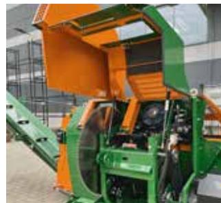
The service area can be accessed without using tools: Saw blades and v-belts can thus be changed quickly and easily.
