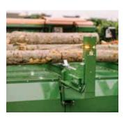
When logs and thus the feed system are starting to move, their movement is visually and acoustically announced via warning lights and a horn.
