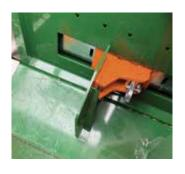
You set the desired billet length yourself (20 – 50 cm) with a single motion and entirely tool-less. Access to the splitting unit is also quick and easy.
