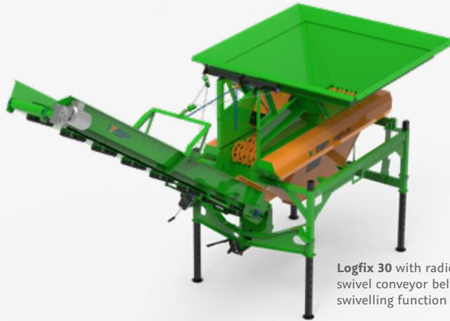
Logfix 30 with radio remote control, swivel conveyor belt 5 m with hydraulic swivelling function and filling funnel
