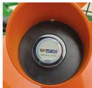
The display indicates pressure, temperature and hour counter as well as wood volume for ease of maintenance and to make and call up settings. Additionally, you can charge your mobile phone at its USB connection.
