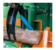
The SuperCut Harvester unit with the 90 cm long blade and the hydraulic double gripper make sure that even the thickest logs are cut safely.
