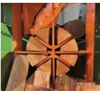
A gradually ascending splitting channel guarantees safe transfer following the cutting process. Splitting stroke optimisation for short logs saves time as the cylinder no longer has to fully extend. This allows you to produce 25% more at billet lengths of up to 33 cm.
