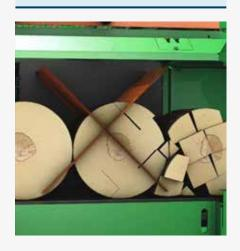
Variability for standardised results. The system with the X-shaped splitting knife produces high-quality firewood in single varieties with the set edge lengths from 5 to 15 cm.
