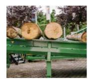
Even crooked and large logs can be processed virtually failure-free as they are separated by segments and thus transported to the cutting unit individually.
