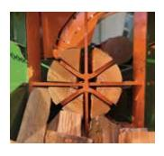
A gradually ascending splitting channel guarantees safe transfer following the cutting process. Splitting stroke optimisation for short logs saves time as the cylinder no longer has to fully extend. This allows you to produce 25% more at billet lengths of up to 33 cm.
