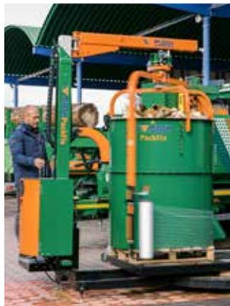
The rotary arm securely wraps the round bale mesh around the filling drum and the billets.
