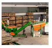
Optionally, the billets that were cut to the required edge length can additionally be cleaned and bagged ready for sale in one working step. Optimise your firewood production with suitable conveyor belts, billet cleaning and bagging solutions from POSCH.
