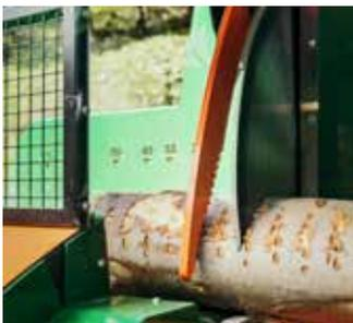
The WIDIA carbide saw blade with 100 cm Ø shortens the log to 20 to 50 cm and is particularly long lasting. The hydraulic log downholder safely retains the logs during the cutting process.
