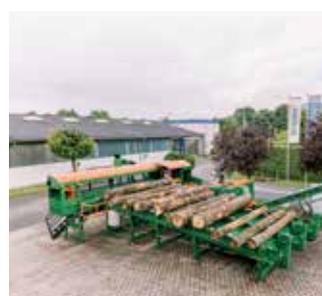
Combined with SpaltFix K-710 a-Vario you can now process up to 17 logs of 70cm Ø in 90 minutes – fully automatically.
