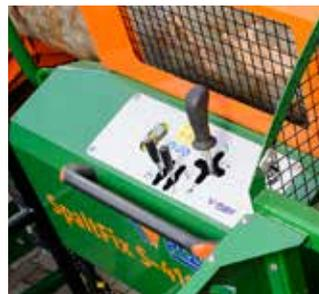
The operator has all processes from charging to cutting directly under control. The optional manipulator makes the positioning of twisted logs easier.
