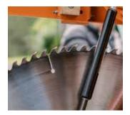
For an increased cutting performance and a longer useful life, a reinforced WIDIA saw blade with a diameter of 90 cm is installed.
