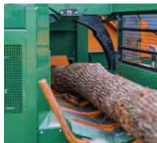
Depending on log volume and log diameter, longitudinal and cross conveyors can be individually combined with each other. The hydraulic log manipulator additionally ensures an optimum log position.
