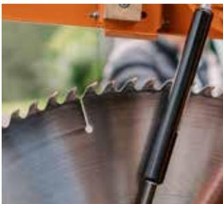
For an increased cutting performance and a longer useful life, a reinforced WIDIA saw blade with a diameter of 90 cm is installed. This guarantees a more quiet and more powerful cutting process.
