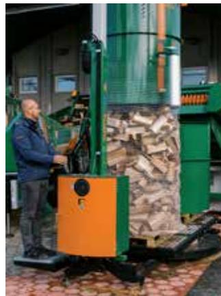
The drum itself does not rotate and is pulled upwards hydraulically.
