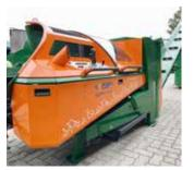
The firewood processor is 100% powder-coated. Its cast pump (formerly aluminium) and the stronger gearbox promise and even longer service life. The valves are electrically controlled, which eliminates the need to replace mechanical wear parts.
