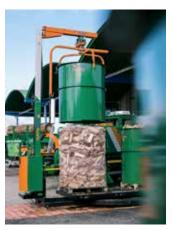
As soon as the filling drum has been pulled up all the way, the mesh is severed and the pack of billets is carted away.
