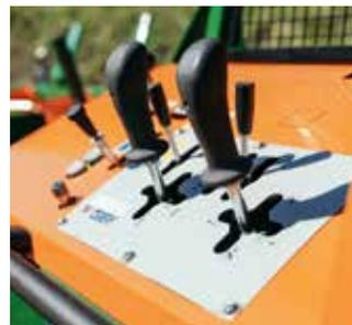
As soon as a log has reached the feeding belt, the cutting/ splitting process can be controlled safely and easily by means of the 2-hand joystick.
