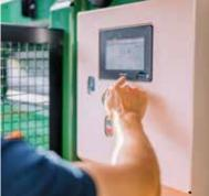
Use the touch screen of the electronic control to adjust the desired cutting length and the admissible length deviations of the finished billets quite easily.
