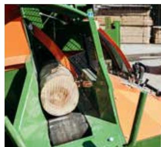
Using the joystick, the log is hydraulically transported to the WIDIA saw blade via a conveyor belt. Log support systems comprising longitudinal and cross conveyors can be combined individually depending on the requirements.
