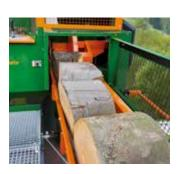
The hydraulic ejection hatch and the standard buffer belt ensure smooth transportation of logs to the splitting process.
