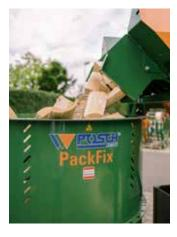
The PackFix drum is filled with a cubic metre of billets by means of a conveyor belt.
