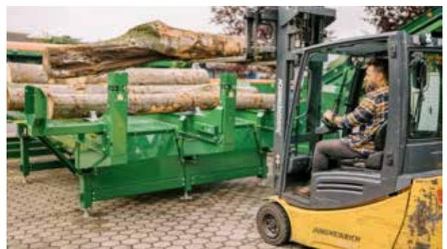
A sheet metal housing around the loading area prevents chips and dirt to accumulate underneath. Residual wood can be collected more easily.
