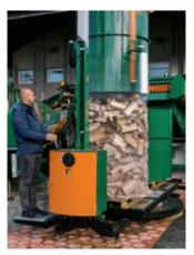
The drum itself does not rotate and is pulled upwards hydraulically.
