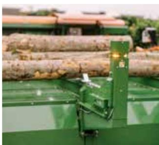
When logs and thus the feed system are starting to move, their movement is visually and acoustically announced via warning lights and a horn.
