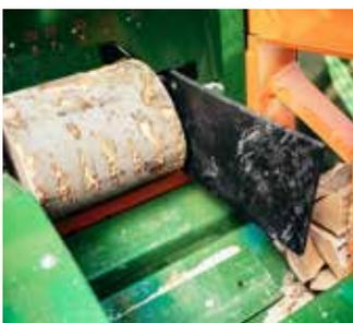
The entire log section is transported to the splitting punch via the hydraulically operated wood rocker. The punch pushes the log against the splitting wedge.
