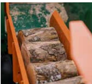
The buffer belt's stop is 2-way adjustable, allowing for operationally safe wood transfer.
