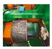
The pressure piece presses the timber with 35 t against the double-edged splitting knife and so quickly produces the maximum number of billets.
