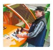
With the 2-hand joystick on the clearly structured control panel, it is easy to control all processes. The log manipulator is used to put the logs in the right position before processing.
