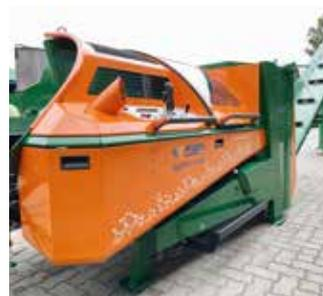
The firewood processor is 100% powder-coated. Its cast pump (formerly aluminium) and the stronger gearbox promise and even longer service life. The valves are electrically controlled, which eliminates the need to replace mechanical wear parts.
