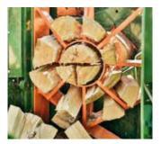
The hydraulically adjustable MULTI frame splitting wedge can be adapted to the log diameter comfortably and produces 2, 6 or 12 billets per work step without having to change the wedge.
