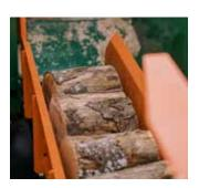
The buffer belt's stop is 2-way adjustable, allowing for operationally safe wood transfer.
