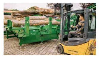
A sheet metal housing around the loading area prevents chips and dirt to accumulate underneath. Residual wood can be collected more easily.
