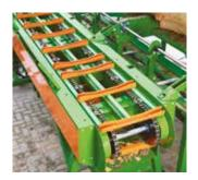
The double chain conveyor with timber manipulator ensures a constant processing speed. Combined with a log support system, you can produce more cubic metres per hour.
