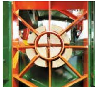
The hydraulically adjustable MULTI splitting knife produces an optimum result with every log diameter. In that way, the machine produces up to 18 same-sized billets per work cycle.
