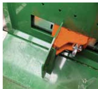
You set the desired billet length yourself (20 – 50 cm) with a single motion and entirely tool-less. Access to the splitting unit is also quick and easy.
