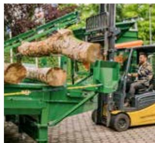
Feeding is possible at all times, even in automatic mode. The system simply reverses rapidly, stopping in the correct position. Several sensors monitor the automated feed process, log transfer and measurement.
