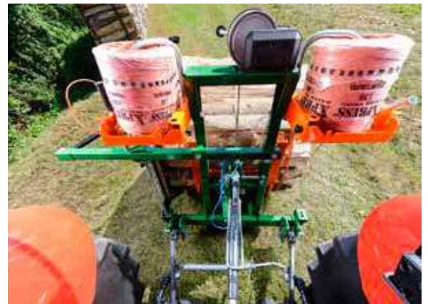
Pressed-yarn cord bundling device is easy to handle and to dispose of.
