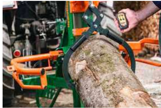
The rope winch with optional gripping pliers and radio remote control for the easy transportation of heavy logs.
