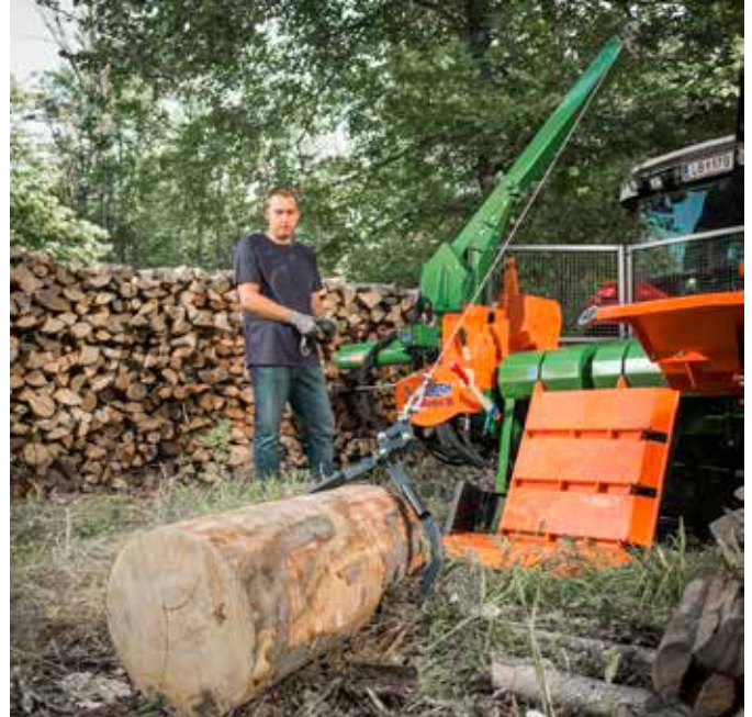
The optional rope winch helps you process even very large logs with ease.
