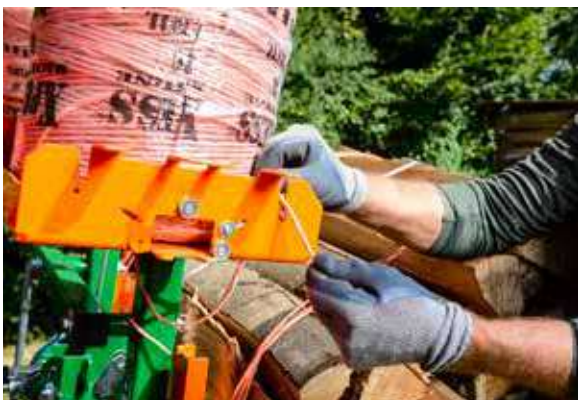
The last step is to knot the yarn and cut it with the integrated cutting device.
