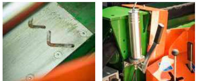
Integrated lubrication device with hand pump (optional).
