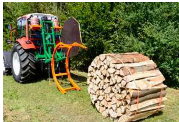
The ready-tied bundle can be conveniently rolled out of the bundling device.
