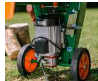
The powerful 5.5 kW e-motor in detail. Here you can also see the parking device for the splitting wedge on the back.
