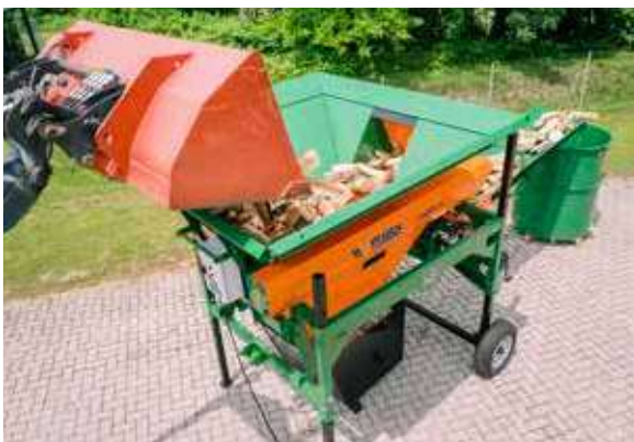
LogFix 30 (formerly LogFix L): Waste wood is transported to a suitable container or an optional conveyor belt. Design with radio remote control (RC), hydr. swivelling conveyor belt (SF3 & H), filling funnel (T) and chassis (F0004723).
