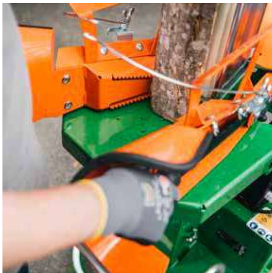
The SpaltAxt 6's automated timber fixation system allows for comfortable and safe splitting.
