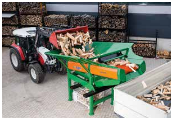
LogFix 60 (formerly LogFix XL): The powerful log screen for large volumes of timber.
