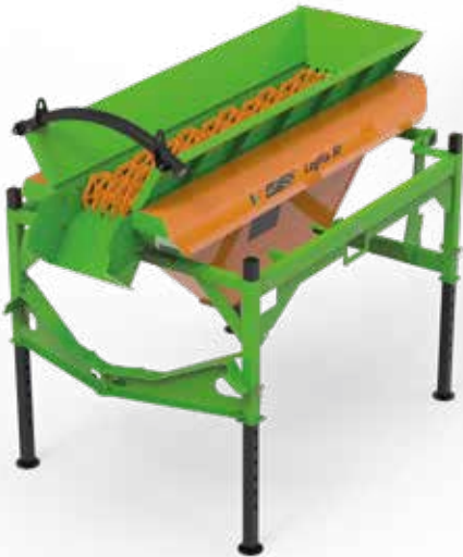
LogFix 30 , can be combined with firewood processors or SpaltFix models. Shovel feed possible with optional funnel. Performance of up to 30 m 3 / h.
