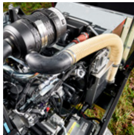
Hatz 4H50 Stage V motor van 55,0 kw
